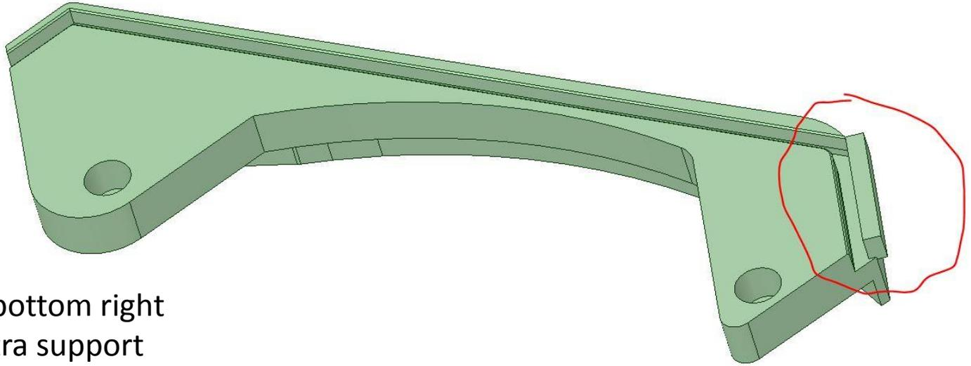
Bottom left and bottom right parts have an extra support designed into them to help printing. This needs to be trimmed off after printed.
